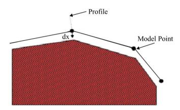
Fig. 5. Suggested movement of point is along normal to boundary, proportional to maximum edge strength on normal.
