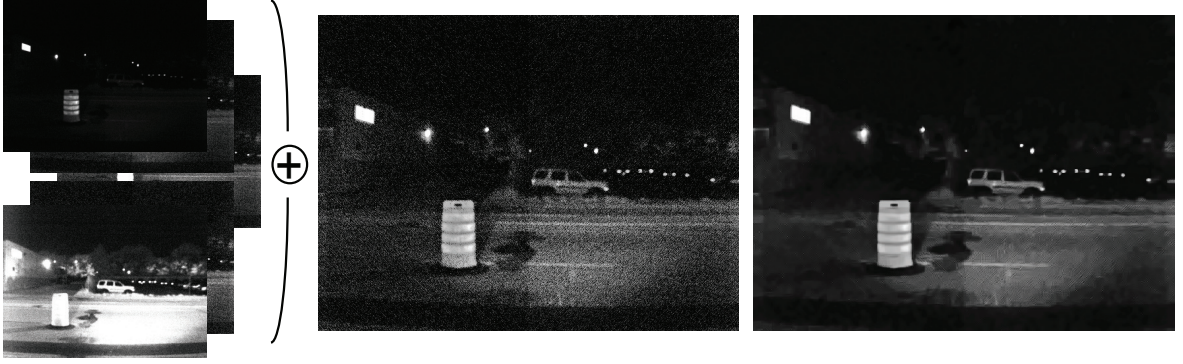
Figure 5.2: The preprocessing of low-light images. (left) A set of images with different exposure time synthesized from a typical HS-M image captured under low-light conditions. (center) is our preprocessing result of the input HS-M image. Notice that the intensity level of dark regions has been boosted while the bright regions are still well under saturation. (right) shows the BM3D denoising result of the preprocessed HS-M image.
