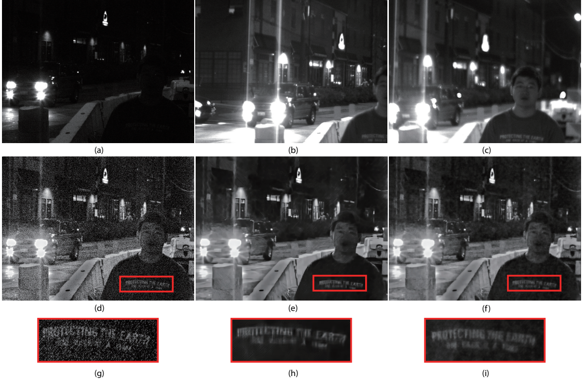
Figure 5.9: Multispectral denoising of an outdoor scene. (a) is a low-light image captured by camera HS-M 0 , and (b)(c) are large aperture stereo images from HR-M cameras. (d) is the preprocessed image from (a), and (e)(f) are the denoising results of (d) by BM3D and our multispectral denoising algorithm respectively. (g-i) are zoomed-in regions of the corresponding rectangle regions shown in (d-f). (The subject depicted here is the author of this thesis.)
