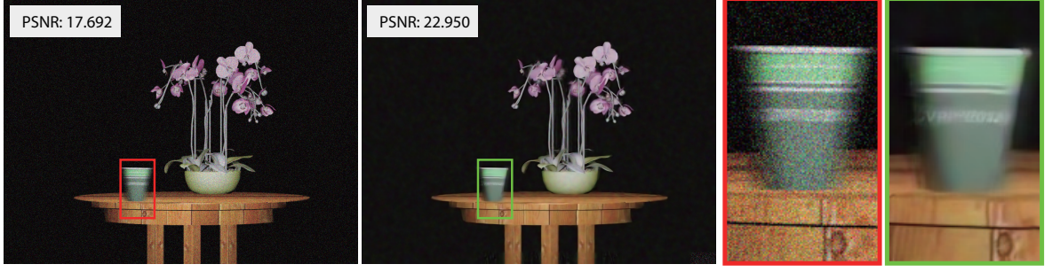
Figure 7.5: Image deblurring/denoising of a synthetic HR-C image. (left) shows the synthesized HR-C image. (center) our deblurring/denoising result. (right) shows the zoomed-in figures corresponding to the rectangle regions in (left) and (center) respectively.
