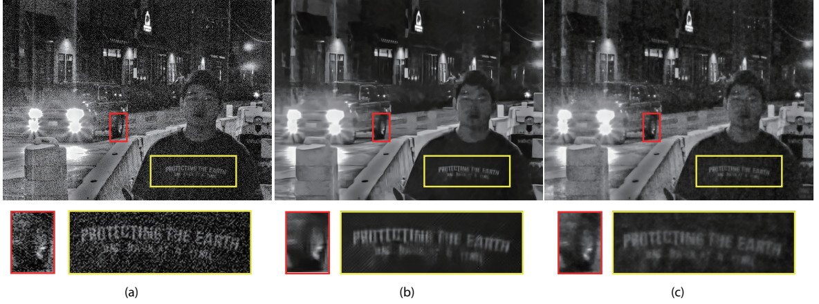
Figure 5.10: Multispectral denoising of the same outdoor scene as Fig.5.9 for the other HS-M camera. (left) the preprocessed low-light image from the second HS-M camera. (center) the BM3D denoising result. (right) our multispectral denoising result. The second row shows zoomed-in regions of the corresponding rectangle areas in the first row. (The subject depicted here is the author of this thesis.)
