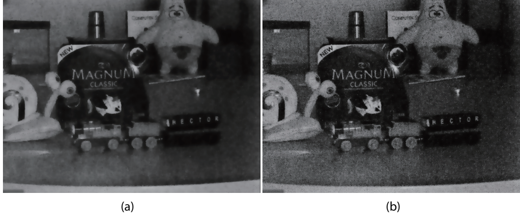
Figure 5.11: Comparison between total variation (TV) denoising and patch based TV denoising. (left) TV denoising result of Fig.5.7(d). (right) patch based TV denoising result.
