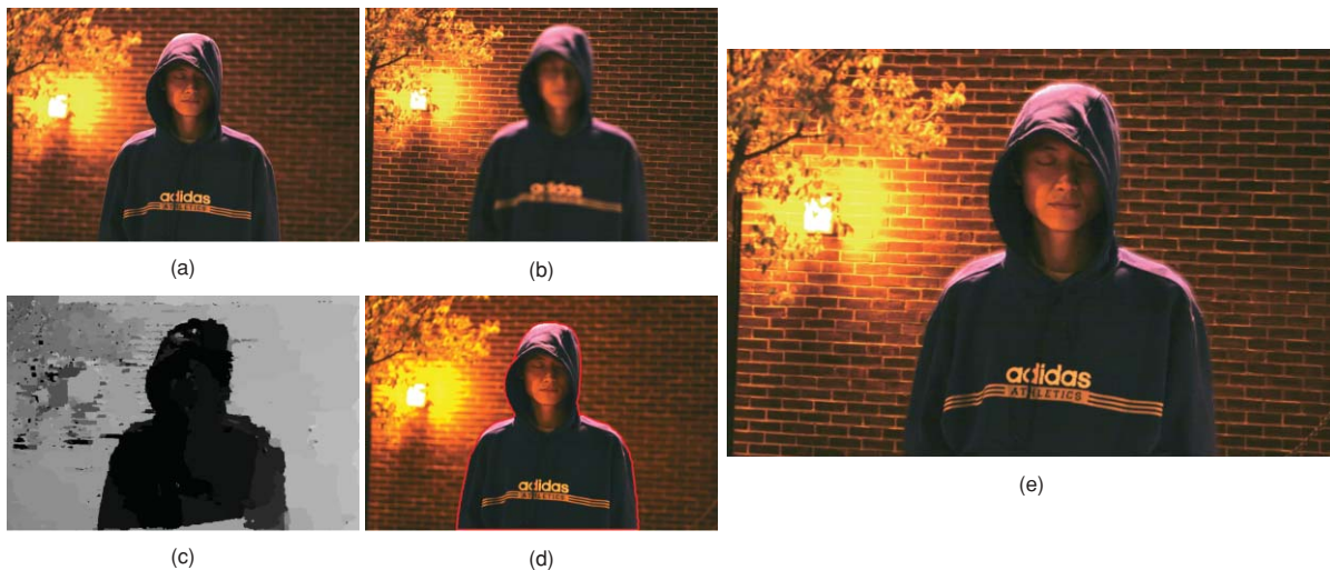
Fig. 7 DFSI for low-light imaging. (a) and (b) show a DFSI pair. We use (c) the DKM to segment the in-focus regions (d) in the first image. Finally, we warp the segmented in-focus regions to the second image using the estimated disparity map to form a nearly all-in-focus image in (e).
