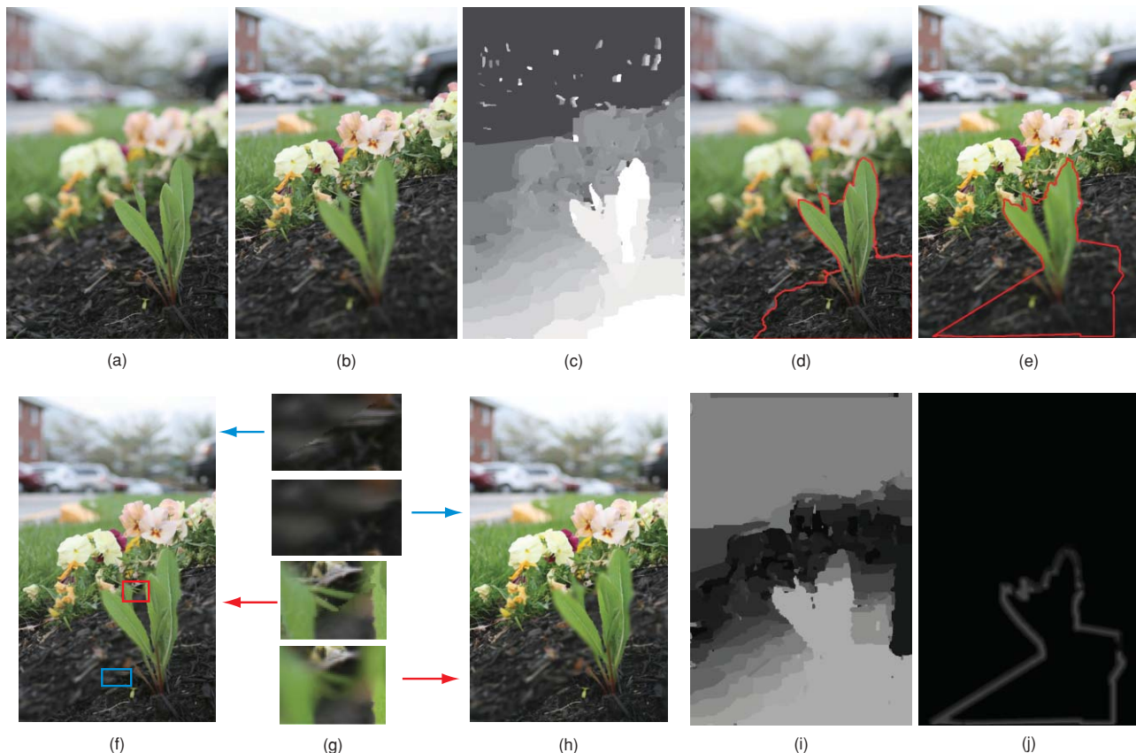
Fig. 10 A multifocus photomontage on a continuous scene. (a) and (b) show a DFSI pair of a garden scene. The first image focuses on the foreground sprouts and the second on the middle-ground flower. (c) and (d) are the recovered disparity map and the segmentation result. (e) shows the warped boundary using the Snake-based algorithm. (f) shows the fusion result by directly warping the segmented foreground to the second image. Notice that the blurriness changes abruptly across the boundary in (g). (h) maintains a smooth boundary by blurring the segmentation boundary using (j) the adaptive kernel map and (i) the DKM.
